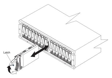
Figure 18. Removing an E-DDM CRU
